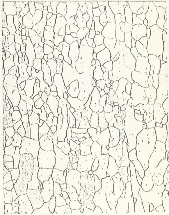
FIG.11 AT 540°C FOR 30 HOURS (ROCKWELL 30T 33.7) -150X- FIG.12 AT 540°C FOR 329.6 HOURS (ROCKWELL 30T 28.8)
